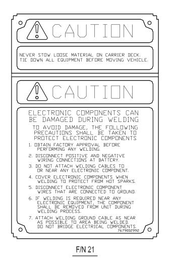
Figure F-1. Location/Description of Signs/Decals/Data Plates (Sheet 15 of 30)
